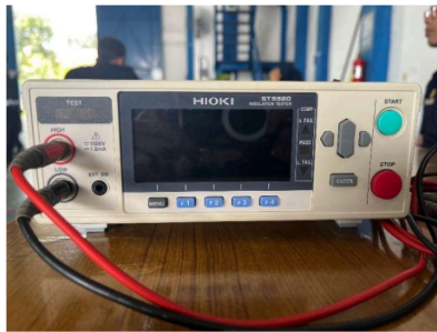
Gambar 11 Alat Uji Insulation
