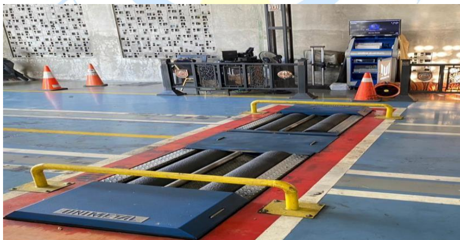
Gambar 2. Alat uji brake tester
