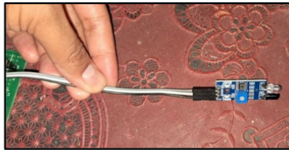
Gambar 33. Perakitan Sensor Infrared FC-51
