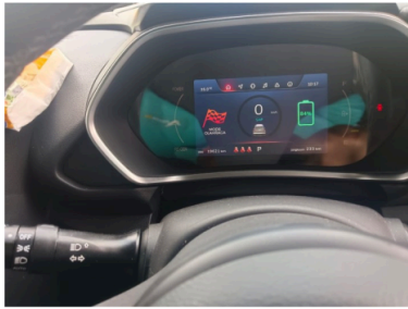
Gambar 36. Memeriksa indikator active driving possible mode
