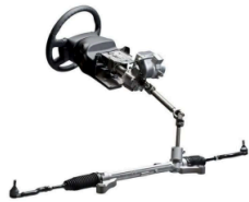
Gambar 2. Sistem kemudi rack and pinion (Sumber: otobltz.net)
